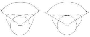
lobe separation = (intake centerline + exhaust centerline)/2
