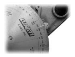
**9** View the degree wheel at this time. This point is 0.050" of lift on the opening side of the intake lobe before top dead center.
