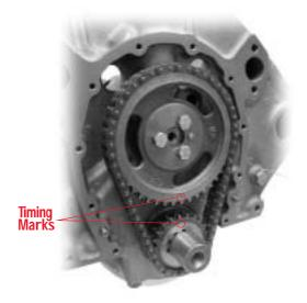
The first step is to install your new camshaft and line up the stock timing marks.
