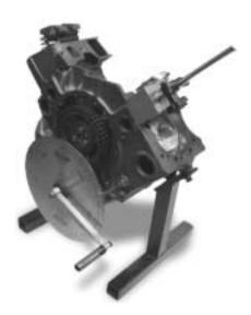
2 To begin the actual degreeing procedure, the degree wheel should be attached to the front of the crankshaft. A pointer of some type such as a piece of wire should be secured to the front of the engine. The engine should be capable of turning in either direction. Use a crank socket or other suitable tool to rotate the engine. At this point you will leave the wheel somewhat loose.
