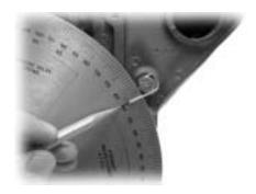
Rotate the engine clockwise until the piston contacts the stop. At this point you should mark the degree wheel.
