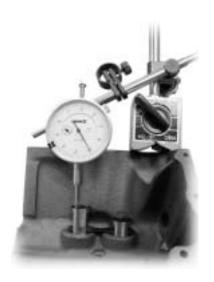
Rotate the engine in clockwise direction until a 0.050" reading is reached.
