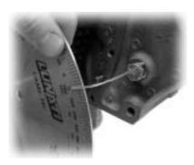
Rotate the crankshaft until the number one piston is at approximate Top Dead Center and align the pointer with TDC on the degree wheel. Tighten the wheel.
