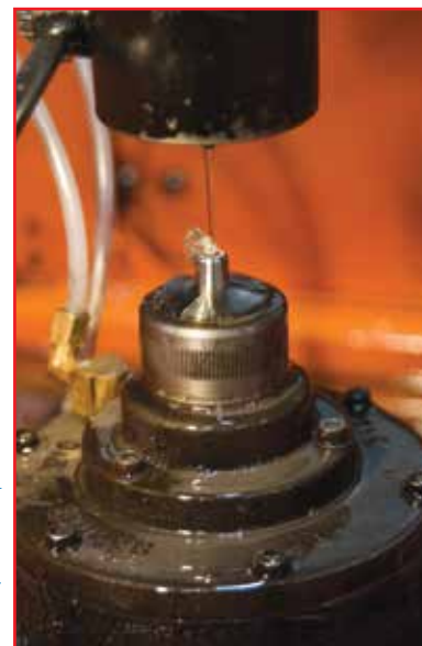
Contemporary EDM technology is used to perform special operations, such as hex-broaching the nose of a unique short-run fastener.
