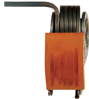
A cam tensioner from an engine that used Royal Purple after an initial break-in period of 1,500 miles.
